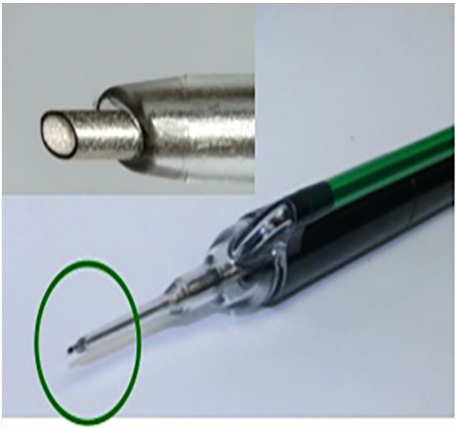
Figure 3: The TX1 ultrasonic treatment device: note the hollow probe that allows aspiration of the diseased tissue. The probe is cooled by a continuous flow of saline that is activated by the ultrasonic energy.
